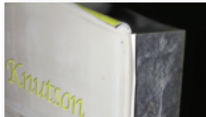
3M™ Sandblast Stencil Tapes offer the durability and consistent thickness that is required when blasting marble or granite.
