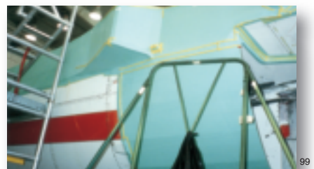
Abrasion-resistant rubber backing and acrylic adhesive of 3M™ Impact Stripping Tapes protect surfaces during plastic media blasting.
